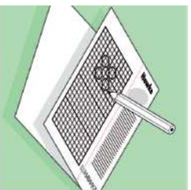
1 Draw up a Hawke Design Template to determine your cable/pipe layout.
