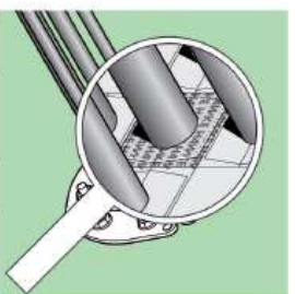
8 Hawke's unique colour coding system enables the installation to be visually inspected after completion and ensures the correct matching of the block halves.
