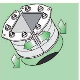
3 Insert the Round Transit Frame and open the two front plate*. No lubricant should be applied to the aperture or outside of the frame
